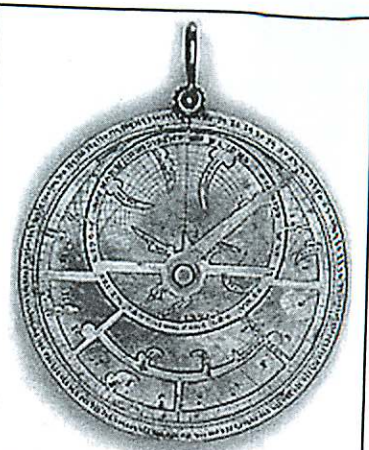
Figure 16. Hispano-Moorish astrolabe, c. 1260, made of brass and copper. Each part of the astrolabe has a central hole so the parts can be held together with a pin and wedge. Parts include plates engraved to indicate the inhabitable regions of the earth; the rete, the celestial part indicating important stars; and the mater, a brass plate with rim. Inventory no. 43504, Museum of the History of Science, Oxford. Courtesy Museum of the History of Science, Oxford.
