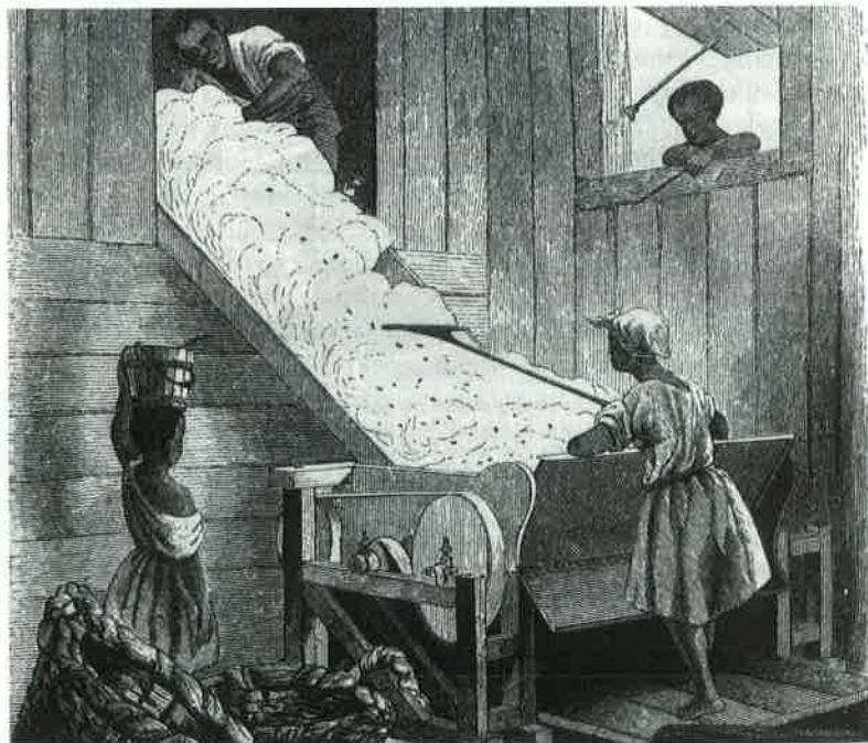
Slaves load cotton into a gin, little changed from Whitney's patent model, in an engraving made in 1854.
